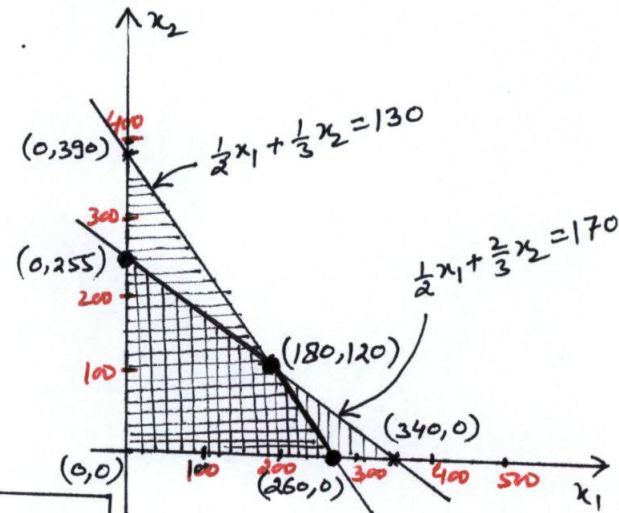
We see that the max. value of  $Z$  is \$520.00 and the corresponding optimal solu. is  $(260, 0)$ . Thus, the candy manufacturer attains maximum sales of \$520 when he produces 260 pounds of mixture A and none of mixture B.
